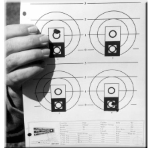
These two three-shot groups were fired with Hornady factory Varmint Express shells loaded with Hornady's 40-grain V-Max varmint bullets.
