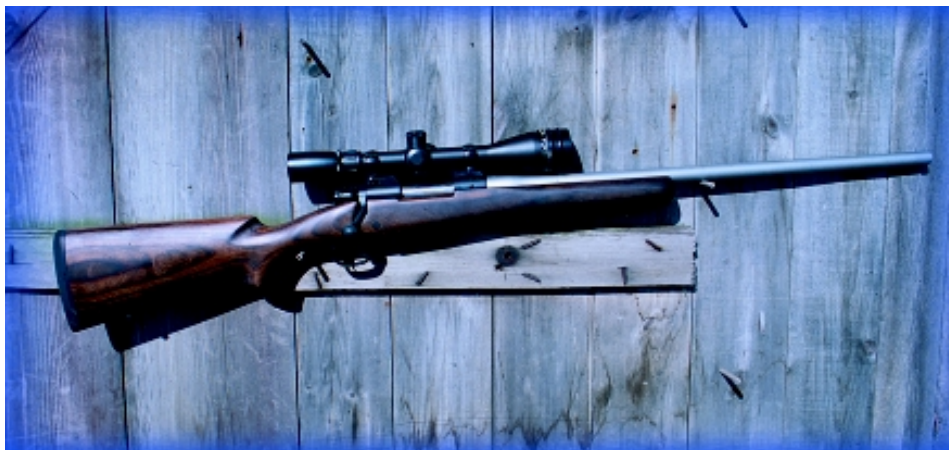
This Winchester Model 70 Coyote rifle in caliber .223 Remington is fitted with a Sightron II 4-16x Mil-Dot scope.
