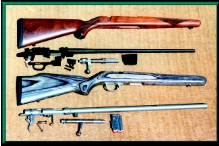
Disassembled views of both .17 HMR rifles. Top rifle is Ruger Model 77/17 with sporter barrel. Bottom rifle is Marlin Model 17VS stainless with 22" varmint barrel.
