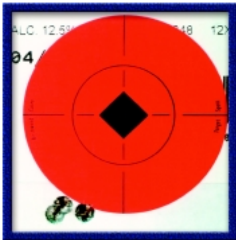
This group was shot from the sitting position at a range of 200 yards, and measures \frac{3}{8} inch.
