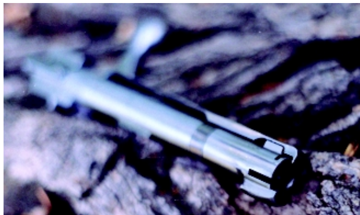
The front of the Ruger Model 77 MKII bolt shows the massive, nonrotating extractor.
