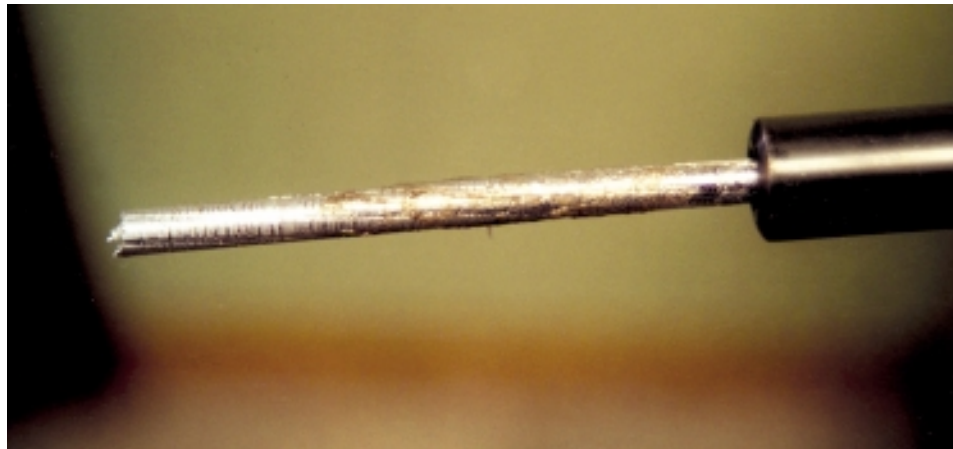
This lead lap was coated with abrasive to smooth the bore.
