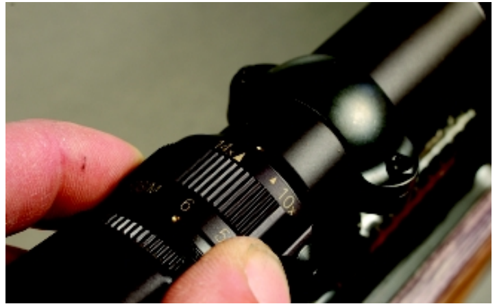
The Varmint Hunter's reticle in the Leupold 4.5-14x50mm scope works when the scope is set on 14x.
