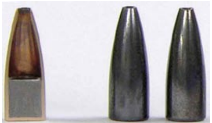
Left: cross-section of 30-grain Berger HP showing the unusually short core. Right: 30- and 40-grain Berger HP, demonstrating that only the core differs — the slight visual difference in nose length, and resulting meplat diameter, is typical of what is commonly seen in nominally identical HP bullets. Berger makes many similar sets of bullets of different weight by using different cores with the same jackets and forming die.
