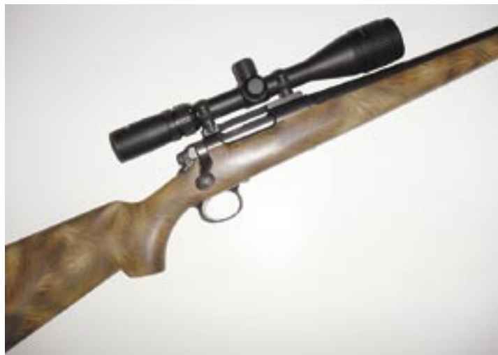
The author used a Remington XP-100 pistol action and a Remington barrel in 223 to build this rifle in 1982. Scope is a Tasco 2.5-10x with mil dot reticle.
