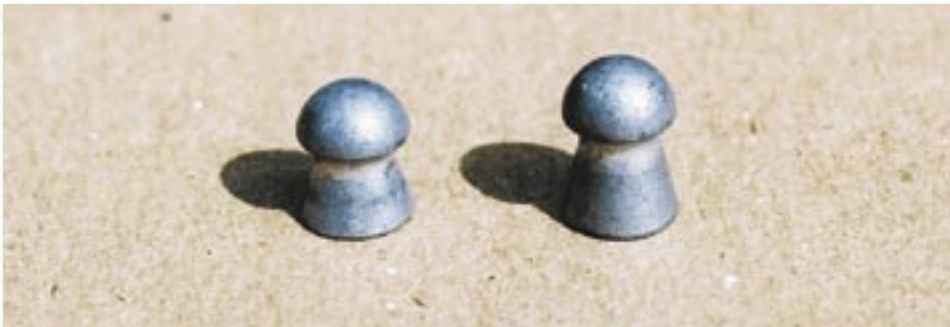
Note the difference in the 7.9-grain and 10.5-grain Crosman Premiers in 177 caliber.
